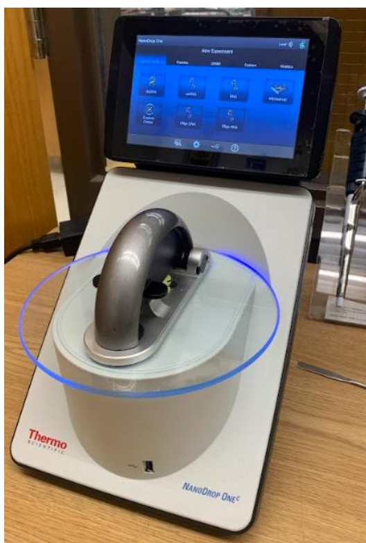
Figure 2: Nanodrop instrument used to measure absorbance at 562nm.
